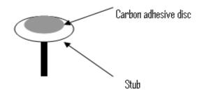
Figure 2. Environmental scanning electron microscope stub.
