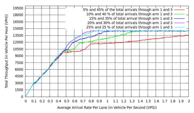
Figure 4. The effect of unbalanced traffic flow at the entrance of a double-lane roundabout. This figure shows the effect of unbalanced traffic volume at entrance road of a roundabout on performance. In this figure traffic volume at arms 2 and 4 are assumed to be each 25% of the total. The rest 50% is distributed unequally to arms 1 and 3 as indicated in the legend.
