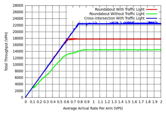
Figure 6. Comparison of roundabout without traffic light, roundabout with traffic light and cross intersection. The figure shows the comparison of roundabout with traffic light and cross intersection. In the simulation the light is assumed to be red for 40 seconds and green for 20 seconds. The yellow time is assumed to be 2 seconds. Every other assumption discussed in this paper also hold true.
