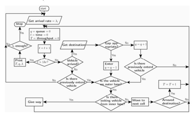
Figure 2.Flowchart of the program used for the simulation.
