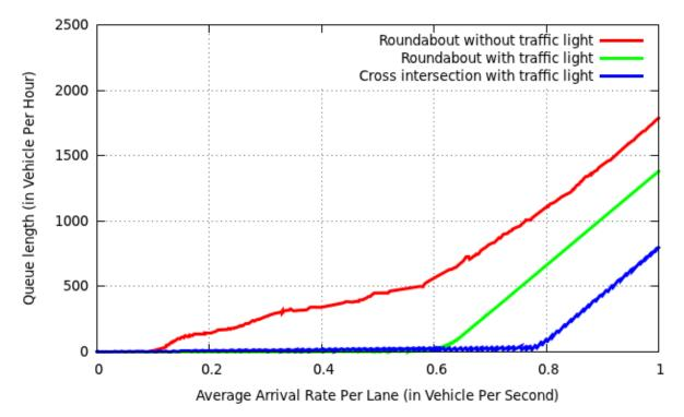
Figure 7. Comparison of the management of Intersection in terms of the queue length formed. The figure shows the comparison of roundabout with traffic light and cross intersection in terms of the queue length formed. Every other assumption discussed in figure 6 also hold true.
