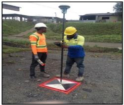
Fig. 6 Survey of Ground Control Point
