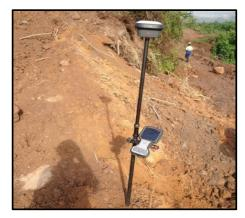
Fig. 2 Leica GPS Receiver
