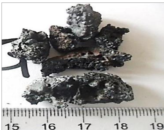
Fig. 7 Samples of Reduced Material obtained after Reduction of 100% Pudo Magnetite Ore with ELT
