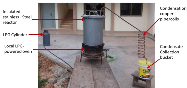
Fig. 3 Locally, Fabricated LPG-Powered Pyrolysis Process Setup
