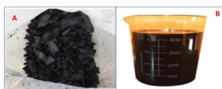
Fig.4 (A) Bio Char and (B) Pyrolysis Oil Produced From Decomposition Process
