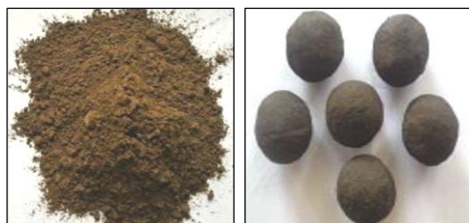
Fig. 5 Spherical Pellets formed from Milled Slag Sample and WES
