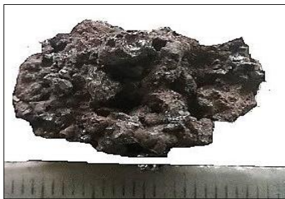
Fig. 19 Reduced Iron formed from Ore after Firing
