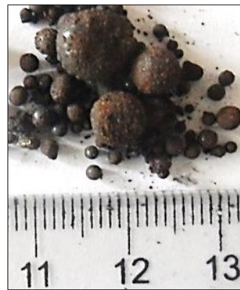
Fig. 15 Samples of Reduced Metal obtained after Reduction at 1550 °C
