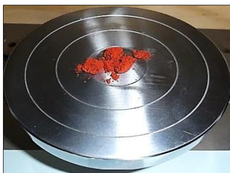
Fig. 5 Appearance of Composite Pellets without Epoxy after Crushing Experiments
