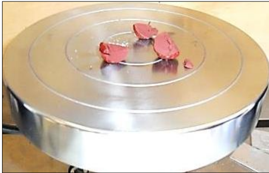
Fig. 4 Appearance of Iron Oxide-Epoxy Composite Pellets after Crushing Experiments
