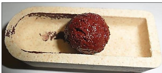
Fig. 1 Iron Oxide-Epoxy Composite Pellet
