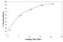
Fig. 6 Grind Analysis of Mill Feed
