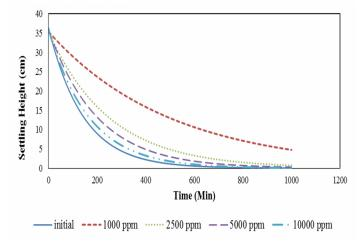
Fig 7 (A) Settling Curves obtained after Deflocculation Test
