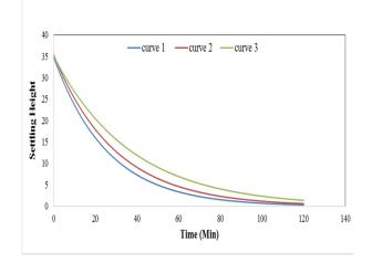
Fig. 3 (C) Thickener Feed Settling Curve. Curves 1, 2 and 3 are Results of Replicates
