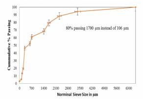
Fig. 1 Screen Analysis of Silt Material
