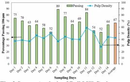
Fig. 2 Screen Analysis of Ball Mill Cyclone Overflow
