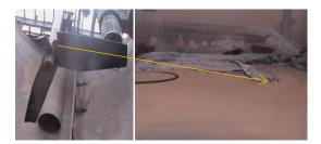
Fig. 5 Mechanical Failure of an Agitator Blade
