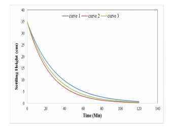
Fig. 3 (A) Ball Mill Cyclone Overflow Settling Curve (BMCO). Curves 1, 2 and 3 are Results of Replicates
