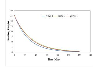
Fig. 3 (B) SAG Mill Cyclone Overflow Settling Curve (SMCO). Curves 1, 2 and 3 are Results of Replicates
