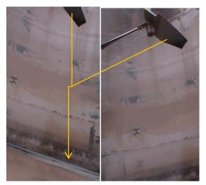
Fig 4 Agitator Off- Bottom
