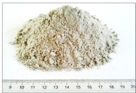
Fig. 1 a) Photograph b) SEM and c) XRD Patterns of Pulverised Carbonaceous Materials Generated from PWS
