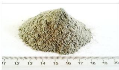
Fig. 2 a) Photograph and b) XRD Patterns of Pulverised Carbonaceous Materials Generated from PP
