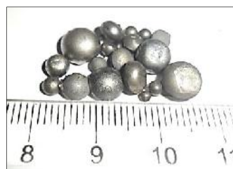
Fig. 8 Nature of Metal Produced from Reduction of Iron Oxide by MPW at 1520 °C
