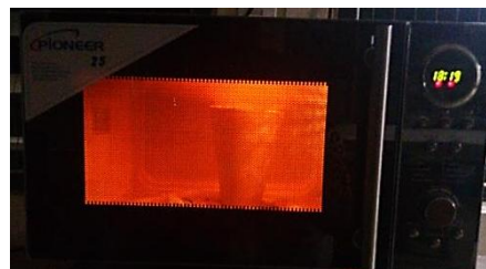
Fig. 2 Calcination Process in Domestic Microwave Oven
