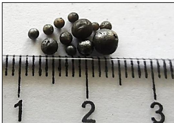
Fig. 10 Droplets of ZnMn 2 O 4 obtained after 1200 Seconds of heating Mn 3 O 4 -ZnO-Graphite-PP Composite
