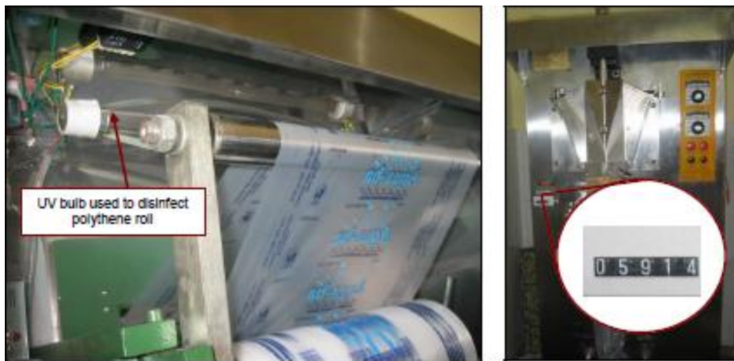
Fig. 4 UV-Bulb in Sachet Water Machine used for Disinfection
