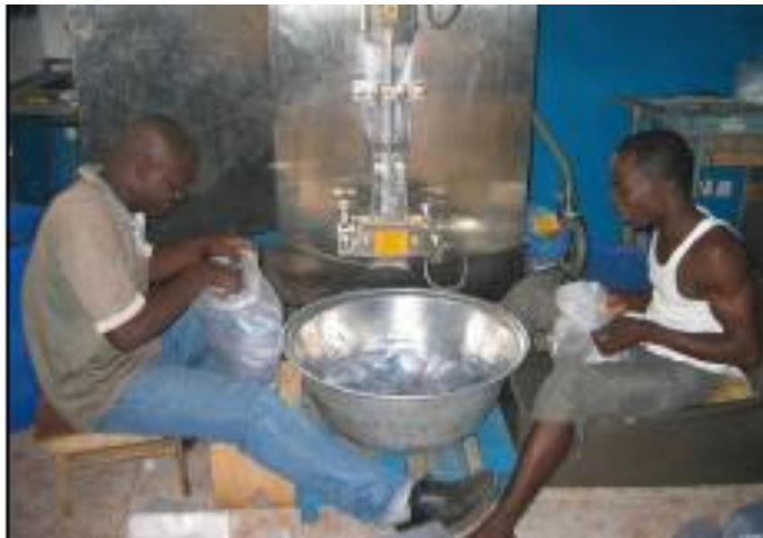
Fig. 2 Bagging of Sachet Water in a Production Area
