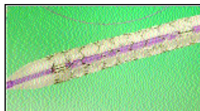
Fig. 5. Coronary artery stent. This photo shows a stent that has been expanded to a diameter of 3 mm by the balloon on which it is mounted. This was a demonstration — the expanded stent can no longer be used and will be discarded.
