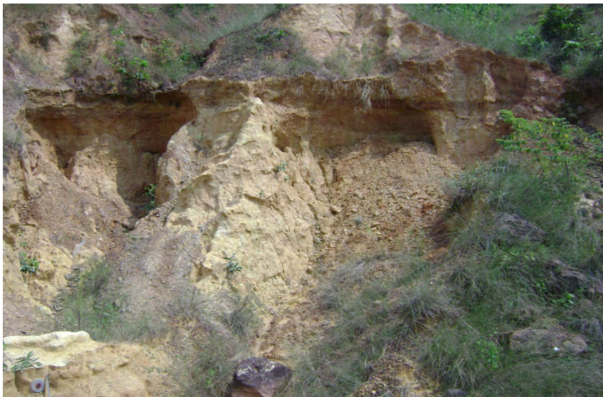
Figure 5 Alcove resulting from basal gully headcut failure in July, 2011. Note the displaced pedon resting at the base of the headcut, the seepage face on the headcut, and the overhanging slope on the top half of the headcut
