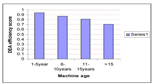
Figure 10: Efficiency score against machine age Index
