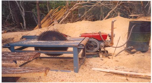
Figure 1: Simple roller-bench mounted on water pump
