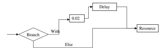
Figure 5 Modelling of failure of a resource
