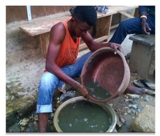
Fig. 14: Extracting gold from the "black" with the aid of mercury at Prestea (Photo by E. Atubouah 2015)
