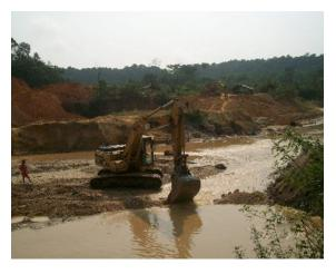
Fig. 6: Miners diverting the course of the river and scooping for alluvial gold (Photo by D. Kumah, 2012)
