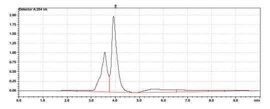
Fig. 6b. Final chromatogramme of insecticide impregnated nets (after their implementation around cages
