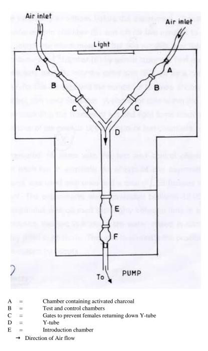
Fig. 1. Diagram of Y-tube olfactometer
