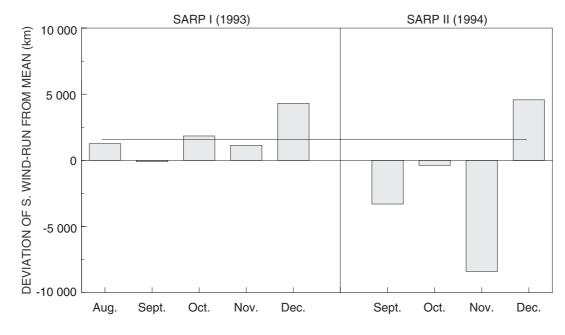
Fig. 2: Monthly deviations of N-S winds from long-term averages (1960–1991) during SARP I and II. The horizontal line indicates the threshold value of 1 667 km
