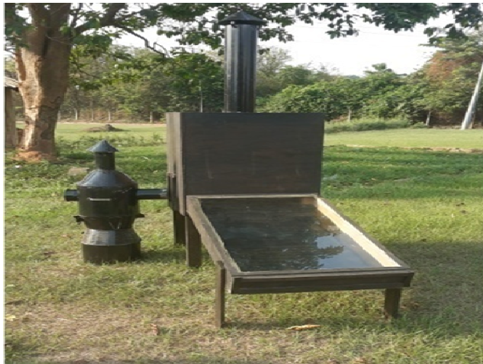
Fig. 2: Experimental set up of the constructed solar dryer with backup heater
