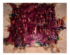
Plate 10: Dyed leather spread out for oxidation to take place
