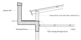
Fig. 5: Parapet Roof with a Downstand beam
