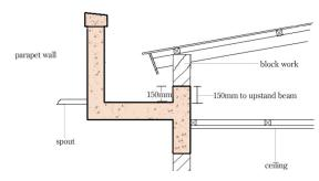
Fig. 9: Use of both an upstand and a downstand beam in a roof gutter.
