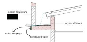
Fig. 6: The use of block work instead of reinforced concrete for a parapet wall
