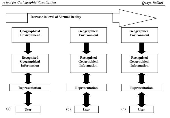
Fig. 1: Schematic illustration of VR regarded as a continuum based upon levels of interaction and the real world; (a) Desktop Virtual Reality where the user can interact with data to vary transformation; (b) Semi-Immersive Virtual Reality where the user is at least slightly immersed by the virtual environment; and (c) Fully Immersive Virtual Reality where the user is fully and physically immersed by the virtual environment (Adapted from Brodlie *et al*, 2002).
