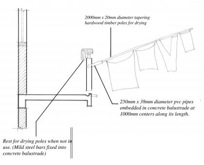
Fig. 8b: Perspective showing the method of drying clothes on upper floors of a multi-storey compound house
