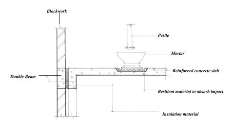
To complement this innovation, voids have been incorporated in the upper floors directly above these areas to accommodate the height of the pestle as it goes up in the pounding process (Fig. 6b). Pounding on the ground floors would be done in the open courtyard, as such none of the modifications in design have been proposed for the households on the ground floor.
