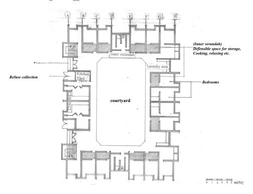
Fig. 5a: Suggested Ground Floor Plan
