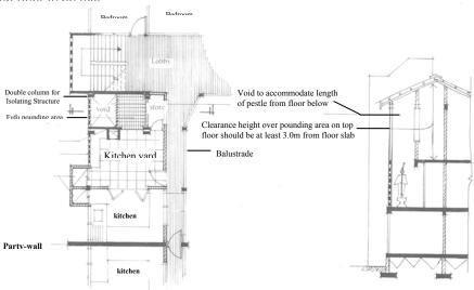
Fig. 6a: Detail of Kitchen/Fufu preparation area on upper floors
