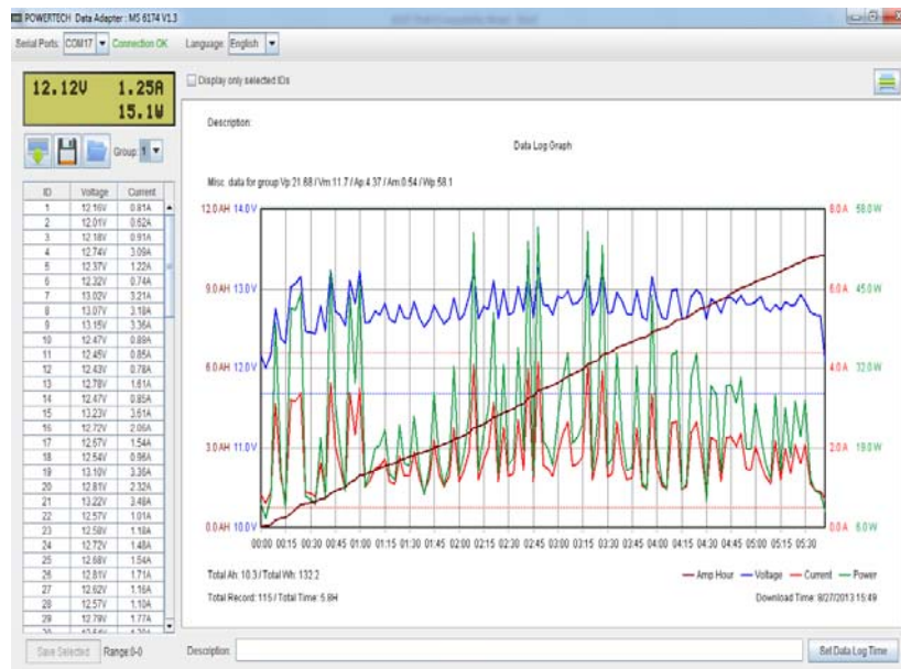
Graph 1. Data Log Graph generated by the applications software using data downloaded in direct cable transmission mode
