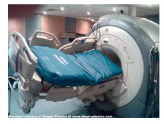
Figure 1: Hospital bed stuck to the inner bore of an MRI magnet – quenching will be the only way to release it
