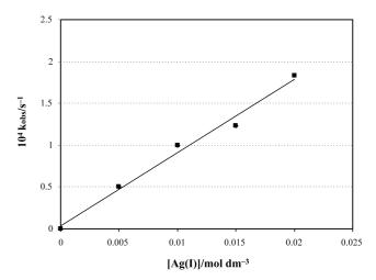
**Figure 5**. Observed first-order rate constant as a function of [Ag<sup>+</sup>] for the  $Cr^{3+}/S_2O_8^{2-}/Ag^+$  reaction.  $[Cr^{3+}] = 0.02 \text{ mol } dm^{-3}; [S_2O_8^{2-}] = 0.04 \text{ mol } dm^{-3}; pH = 2.8 \pm 0.1; T = 40.0 \pm 0.1^{\circ}C.$
