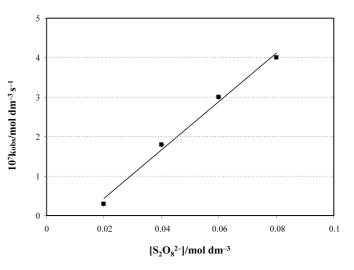
**Figure 6**. The effect of  $[S_2O_8^{2-}]$  on the reaction rate of the  $Cr^{3+}/S_2O_8^{2-}/Ag^+$  reaction.  $[Cr^{3+}] = 0.005 \text{ mol } dm^{-3}$ ;  $[Ag^+] = 0.02 \text{ mol } dm^{-3}$ ;  $pH = 2.8 \pm 0.1$ ;  $T = 40.0 \pm 0.1^{\circ}C$ .
