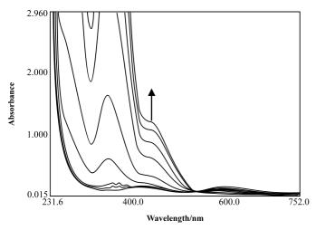
**Figure 1**. Typical absorbance changes observed during the oxidation of Cr(III) by peroxodisulphate induced by silver(I) ion.  $[Cr^{3+}] = 0.02$  mol dm<sup>-3</sup>;  $[S_2O_8^{2-}] = 0.04$  mol dm<sup>-3</sup>;  $[Ag^+] = 0.02$  mol dm<sup>-3</sup>;  $pH = 2.8 \pm 0.1$ ;  $T = 40.0 \pm 0.1^{\circ}C$  (arrow shows direction of change).
