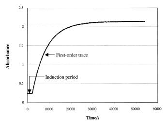
**Figure 2**. Typical kinetic trace for the silver(I)-induced oxidation of Cr(III) by peroxodisulphate at high [Cr(III)]. [Cr<sup>3+</sup>] = 0.02 mol dm<sup>-3</sup>; [Ag<sup>+</sup>] = 0.02 mol dm<sup>-3</sup>; [S<sub>2</sub>O<sub>8</sub><sup>2-</sup>] = 0.04 mol dm<sup>-3</sup>;  $\lambda$  = 440 nm; pH = 2.8 ± 0.1; T = 40.0 ± 0.1°C.
