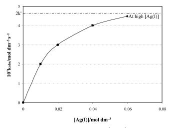
Figure 7. Observed rate constants for the Cr<sup>3+</sup>/S<sub>2</sub>O<sub>8</sub><sup>2-</sup>/Ag<sup>+</sup> reaction as a function of [Ag<sup>+</sup>]. [Cr<sup>3+</sup>] = 0.005 mol dm<sup>-3</sup>; [S<sub>2</sub>O<sub>8</sub><sup>2-</sup>] = 0.1 mol dm<sup>-3</sup>; pH =  $2.8 \pm 0.1$ ; T =  $40.0 \pm 0.1$ °C.
