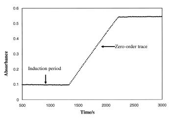
**Figure 3.** Typical kinetic trace for the silver(I)-induced oxidation of Cr(III) by peroxodisulphate at low [Cr(III)]. [Cr<sup>3+</sup>] = 0.001 mol dm<sup>-3</sup>; [Ag<sup>+</sup>] = 0.02 mol dm<sup>-3</sup>; [S<sub>2</sub>O<sub>8</sub><sup>2-</sup>] = 0.1 mol dm<sup>-3</sup>;  $\lambda$  = 440 nm; pH = 2.8 ± 0.1; T = 40.0 ± 0.1°C.
