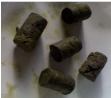
Figure 1. Glycerine pellet produced from waste glycerine and biomass.
