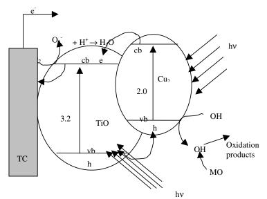
Photoelectrocatalytic removal of color from water using  $TiO_2$  and  $TiO_2/Cu_2O$  electrodes 39
