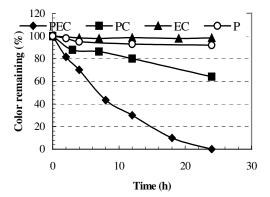
Figure 7. Removal of color by photolysis, photo catalysis, electrolysis, and photoelectrocatalysis (+1.0 V) using TiO<sub>2</sub> electrode in photoelectrochemical reactor.
