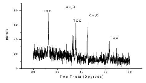
Figure 3. X-ray diffraction patterns of copper oxides deposited at -0.4 V on TCO from alkaline lactate solution pH 10.
