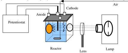
Figure 2. Schematic diagram of photocatalysis and photelectrocatalysis reactor system.
