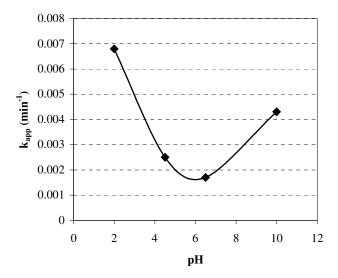
Figure 9. Variation of apparent reaction rate constant as a function of pH at bias potential of +1.5 V using TiO<sub>2</sub> thin film electrode.
