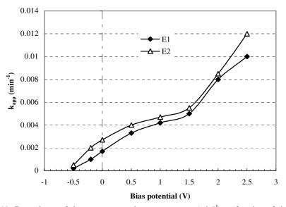
Figure 11. Dependence of the apparent reaction rate constant (min<sup>-1</sup>) as function of time at different potential in  $K_2SO_4$  at pH 10 using TiO<sub>2</sub> thin film electrodes.
