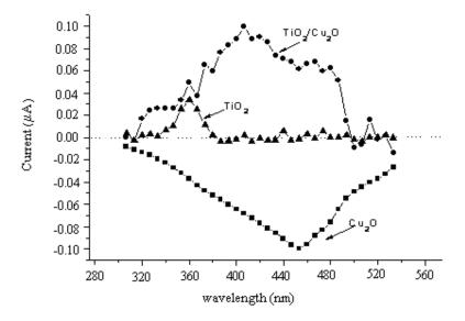
Figure 6. Spectral photo response of the electrodes prepared from alkaline lactate solution at pH 10.
