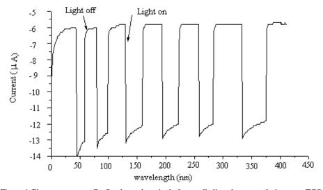
Figure 4. Photo response Cu<sub>2</sub>O electrodeposited from alkaline lactate solution on TCO conduction substrate under oxygen bubbling (0.5 M K<sub>2</sub>SO<sub>4</sub>, 0.2 mA/cm<sup>2</sup>, -0.4 V).
