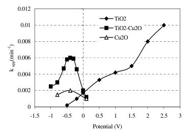
Figure 12. Dependence of the apparent reaction rate constant (min<sup>-1</sup>) as function of time at different potential in  $K_2SO_4$  at pH 10 using Cu<sub>2</sub>O, TiO<sub>2</sub>, and TiO<sub>2</sub>/Cu<sub>2</sub>O composite thin-film electrodes.
