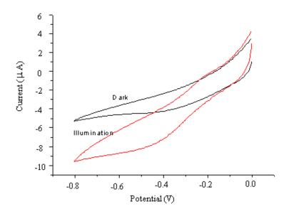
Figure 5. Cyclic voltammogram of Cu<sub>2</sub>O thin film deposited at -0.4 V on TCO from alkaline lactate solution pH 10 (scan rate 10 mV/s., 0.5 M K<sub>2</sub>SO<sub>4</sub> electrolyte).
