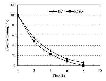
Figure 10. Color removal as a function of irradiation time at pH 2 with TiO<sub>2</sub> thin film electrodes (E1) at bias potential of 1.5 V in KCl and K<sub>2</sub>SO<sub>4</sub> supporting electrolytes.
