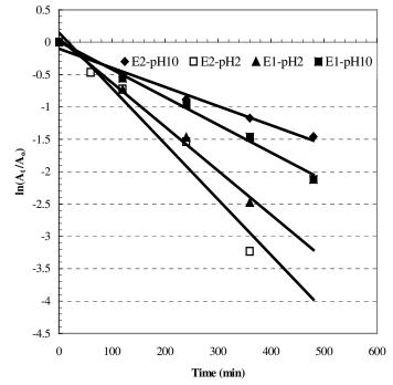
Figure 8. Effect of pH on photoelectrocatalytic color removal at bias potential of +1.5 V using TiO<sub>2</sub> thin film electrodes.
