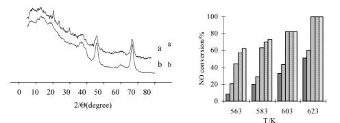
Figure 4. XRD patterns of the catalysts. a: Pt-Rh-Pd/Al<sub>2</sub>O<sub>3</sub> and b: Pt-Rh-Pd-1.56% Cu/Al<sub>2</sub>O<sub>3</sub>.
