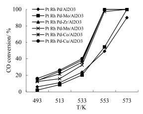
Figure 1. Effect of transitions metal oxides on the catalytic activity for CO oxidation.
