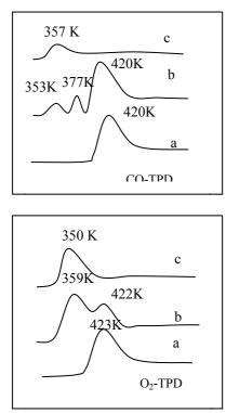
Figure 6. TPD profiles of the catalysts. a: Pt Rh Pd/Al<sub>2</sub>O<sub>3</sub>, b: Pt Rh Pd-1.56% Cu/Al<sub>2</sub>O<sub>3</sub>, c: 1.56%Cu/Al<sub>2</sub>O<sub>3</sub>.
