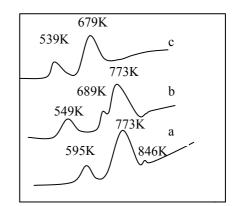
Figure 7. TPR profiles of the catalysts. a: Pt Rh Pd/Al<sub>2</sub>O<sub>3</sub>, b: Pt Rh Pd-1.56% Cu/Al<sub>2</sub>O<sub>3</sub>, c: 1.56%Cu/Al<sub>2</sub>O<sub>3</sub>
