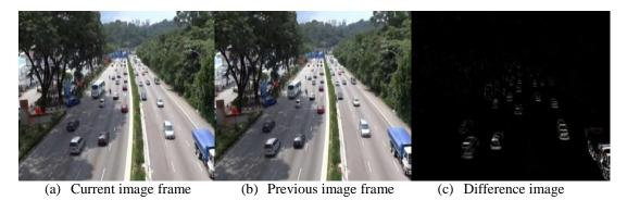
frame **Figure 5:** Modular system testing of the inter-frame vehicle tracking component.
