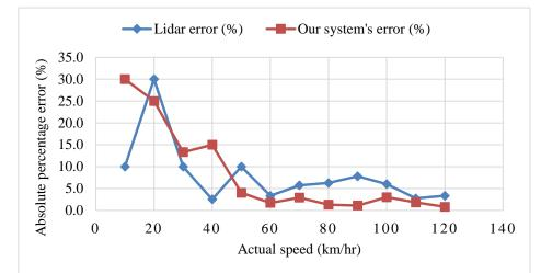
Figure 7: Percentage errors of lidar and proposed systems with frame skipping equals two.
