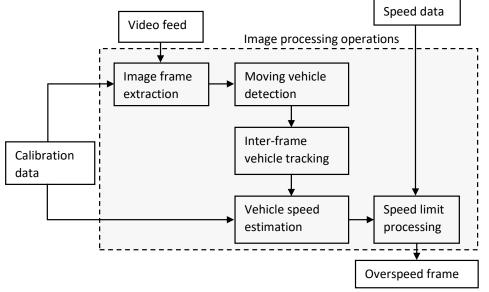
Figure 1: Block diagram of the proposed multi-vehicle speed estimation algorithm.
