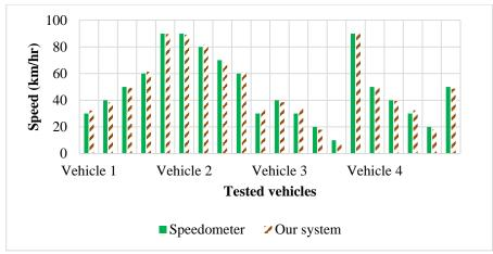
Figure 10: Speed measurements between ideal and proposed systems for different vehicles.
