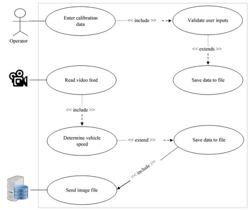
Figure 2: Use Case diagram of the system.
