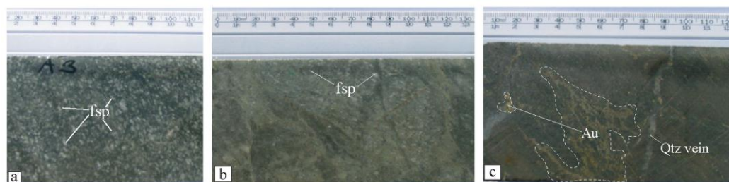
Figure 4: Gokona and Nyabigena andesite (a) Unaltered or weakly altered andesite with clearly visible feldspar phenocrysts, (b and c) strongly altered and mineralised andesite, and (c) decreased amount of feldspar phenocryst in strongly altered andesite and presence of visible gold.
