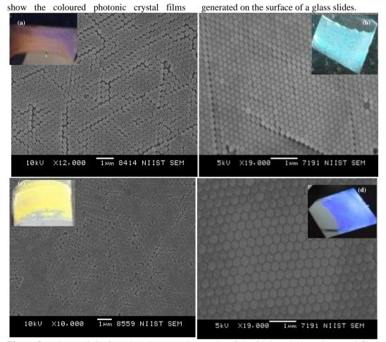
**Figure 3** (a, b, c and d): Scanning electron micrographs of the fabricated photonic crystal films with insets of the obtained photonic crystal films on glass slides.
