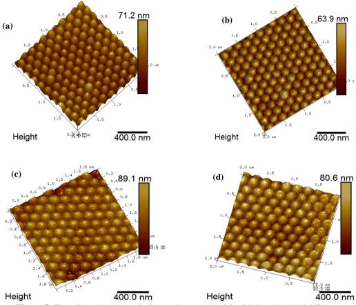
Figure 5: Two-dimensional atomic force micrographs of the fabricated colloidal films.
