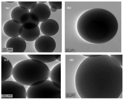
Figure 2: Transmission electron micrographs of (a) 200 nm (b) 130 nm (c) 295 nm (d) 158 nm as-synthesized P(St-MMA-AA) microspheres.
