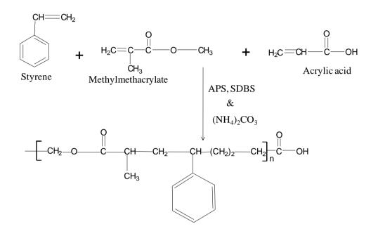
Poly(styrene-methylmethacrylate acrylic acid) Scheme 1: Reaction stages leading to the formation of P(St-MMA-AA) microspheres.
