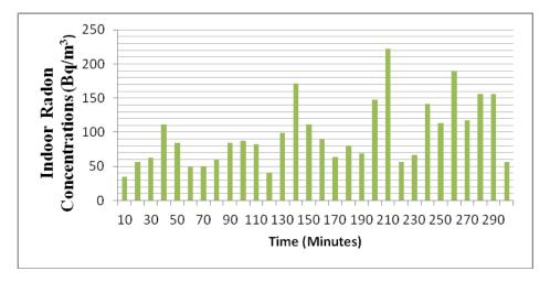
**Figure 3:** Variation of Indoor Radon Gas Concentrations with Time from Kamenyanga Village (H6). Mean Indoor Radon= 96±8 Bq/m<sup>3</sup>
