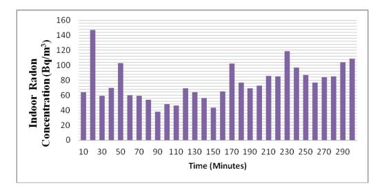
Figure 2: Variation of Indoor Radon Gas Concentrations with Time from Agondi Village (H1). Mean Indoor Radon =  $74\pm 6$  Bq/m<sup>3</sup>
