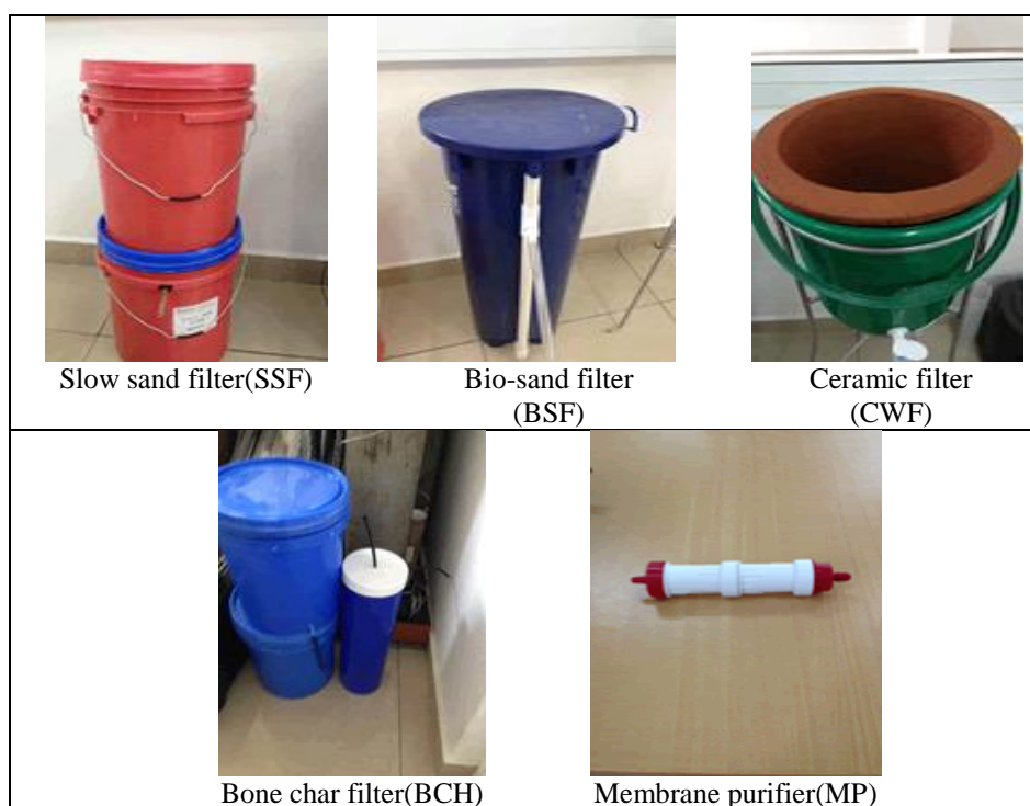
Plate 1: Water filters used for study
