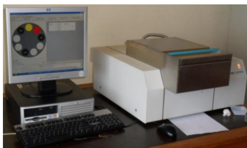
Figure 4: External view of the Spectro Xepos™ EDXRF system.
