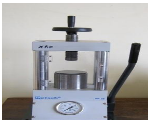
Figure 2: The Retsch™ Press for compressing the powder into a pellet.
