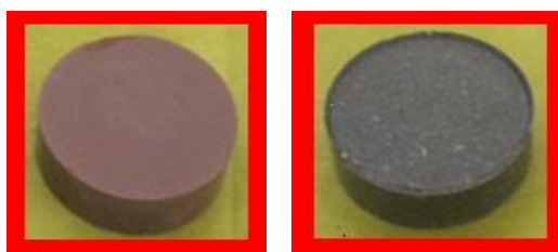
Figure 3: The pellets samples prepared for EDXRF analysis.
