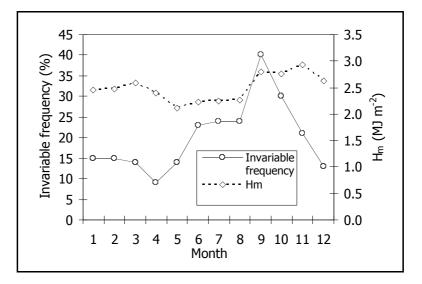
Figure 1: Monthly relative frequencies of the invariable hours and mean monthly hourly global radiation (H<sub>m</sub>).
