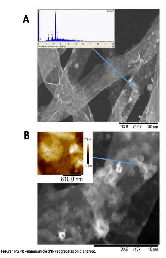
Typical scanning electron microscopy- energy-dispersive X-ray spectroscopy (EDS) images of PGPR cells grown with NPs for 24 hours on plant root after 6 hours of inoculation (**A**). and the characteristic aggregate sizes of 50–60 nm (**B**). Timmusk et al 2018 Nature, SciRep 10.1038/s41598-017-18939-x
