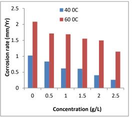
Fig.6: Corrosion rate of Pipeline steel in  $H_2SO_4$  with and without ECB at 40 and 60 °C
