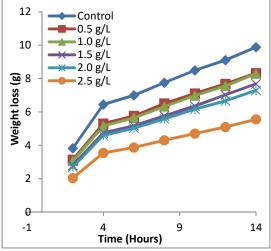
**Fig.3:** Variations in weight loss with time for pipeline steel coupons in 0.5 M H<sub>2</sub>SO<sub>4</sub> solution containing different concentrations of *Enantia chlorantha* at 60 °C
