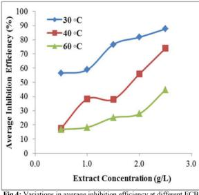
Fig.4: Variations in average inhibition efficiency at different ECB extract in 0.5 M  $\rm H_2SO_4$
