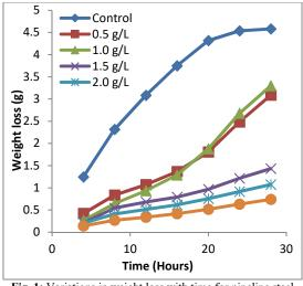
Fig. 1: Variations in weight loss with time for pipeline steel coupons in 0.5 M H<sub>2</sub>SO<sub>4</sub> solution containing different concentrations of *Enantia chlorantha* at 30 °C
