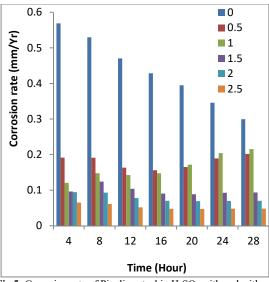
Fig.5: Corrosion rate of Pipeline steel in  $H_2SO_4$  with and without ECB extract at 30 °C
