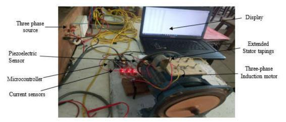
Fig 1. Experimental Test Rig for Data Acquisition
