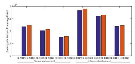
Fig 5. Approximation wavelet energy for healthy and inter-turn current obtained for db4 and db8
