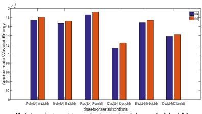
Fig 6. Approximate wavelet energy for phase-to-phase fault current for db4 and db8
