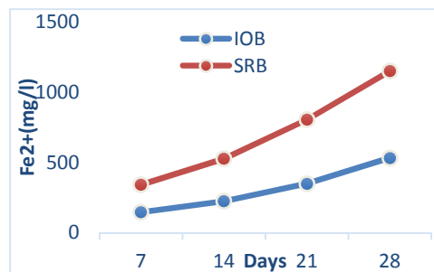
Fig 3: Iron (II) ion ( \text{mg}/\text{l} ) of suspension containing Iron Oxidizing and Sulphur Reducing Bacteria
