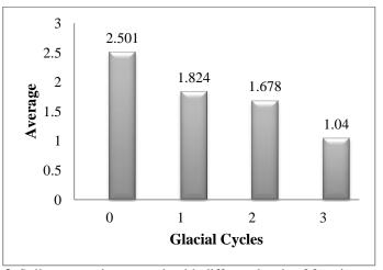
Fig 3. Soil compressive strength with different levels of freezing cycles
