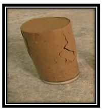
Fig 1. Sample with 1.5% of nanoclay under one freezing cycle
