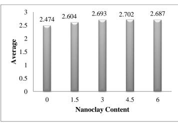
Fig 2. Soil compressive strength with different percents of nanoclay
