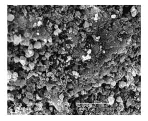
Fig 2: Scanning electron micrograph of bone char particles with 5000X magnifications
