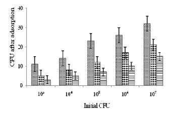
■4g  $\blacksquare$ 7g  $\equiv$ 10g Fig 5: Effect of amounts of BC on adsorption of *E. coli* by the BC >40 mesh
