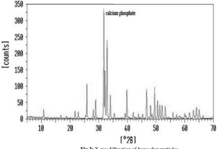
Fig 3: X-ray diffraction of bone char particles
