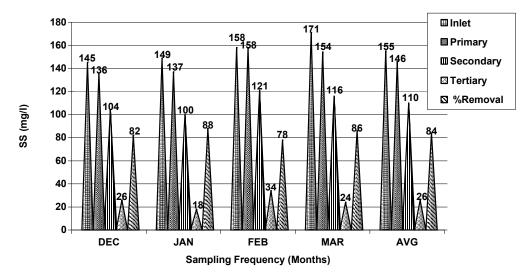
Fig 3: Status of Suspended Solids (SS) at different treatment levels of CETP
