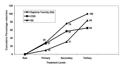
Fig 4: Cumulative reduction of performance parameters at different treatment levels of CETP
