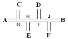
Fig. 2:  $\mu$ FIA manifold for determining flow characteristics of reagents (channels: 200  $\mu$ m wide, 50  $\mu$ m deep). A = reagent reservoir, B = waste reservoir and C-F = side channel reservoirs. AB = 18 mm, AG = GH = HI = IJ = JB = 3.5 mm, CG = EH = DI = FJ = 8 mm.
