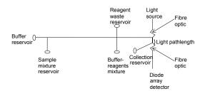
Fig. 5: On-chip manifold for procedure (ii).
