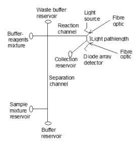
Fig. 4: On-chip manifold for procedure (i).
