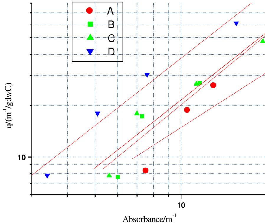
**Figure 4.** Freundlich adsorption isotherm lines for UV<sub>254</sub> of the GAC samples at different heights of the biofilter. A, B, C and D: BAC samples taken from different heights of the biofilter; at 0.25, 0.45, 0.65 and 0.85 m, respectively.
