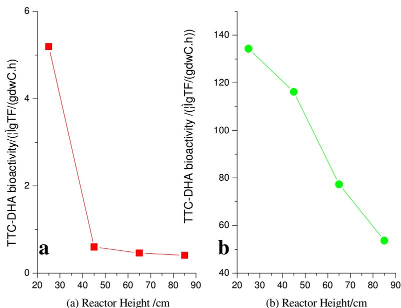
**Figure 2.** Comparison between TTC-DHA bioactivities determined by (a) conventional and (b) modified measurement methods in attached biofilm bioactivity determination with the same batch BAC samples at different heights of the biofilter.
