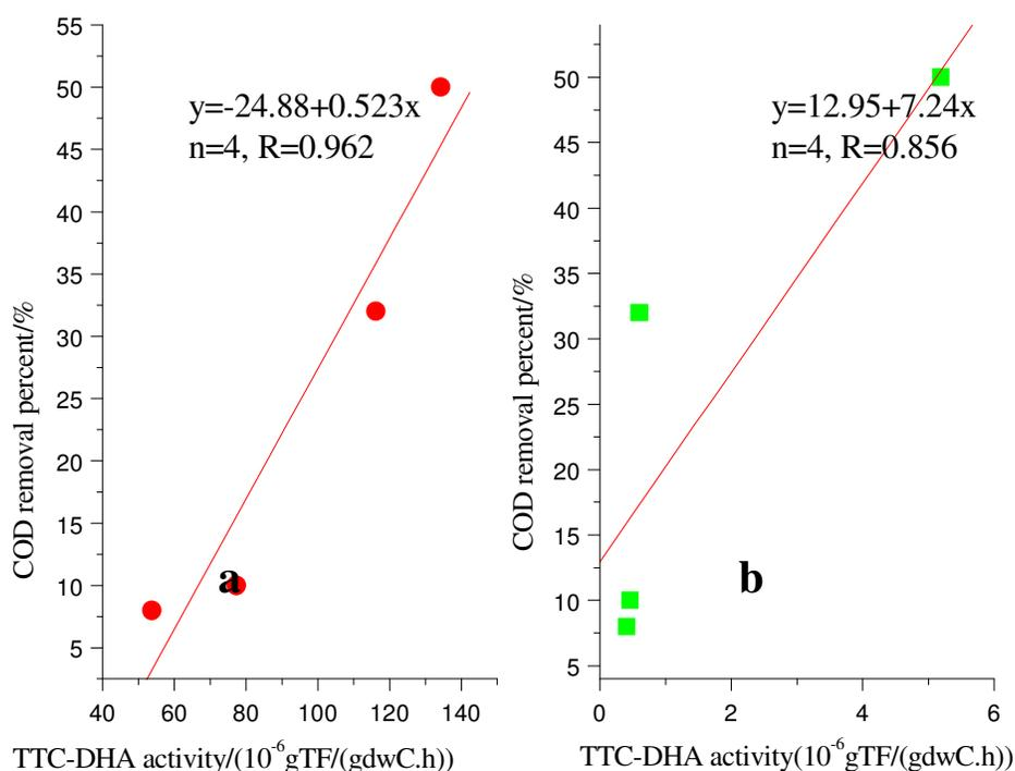
**Figure 3.** Correlations between COD removal proportions and bioactivities at different height sections of the biofilter: **a.** TTC-DHA activities determined in modified way. **b.** TTC-DHA activities determined in conventional way.
