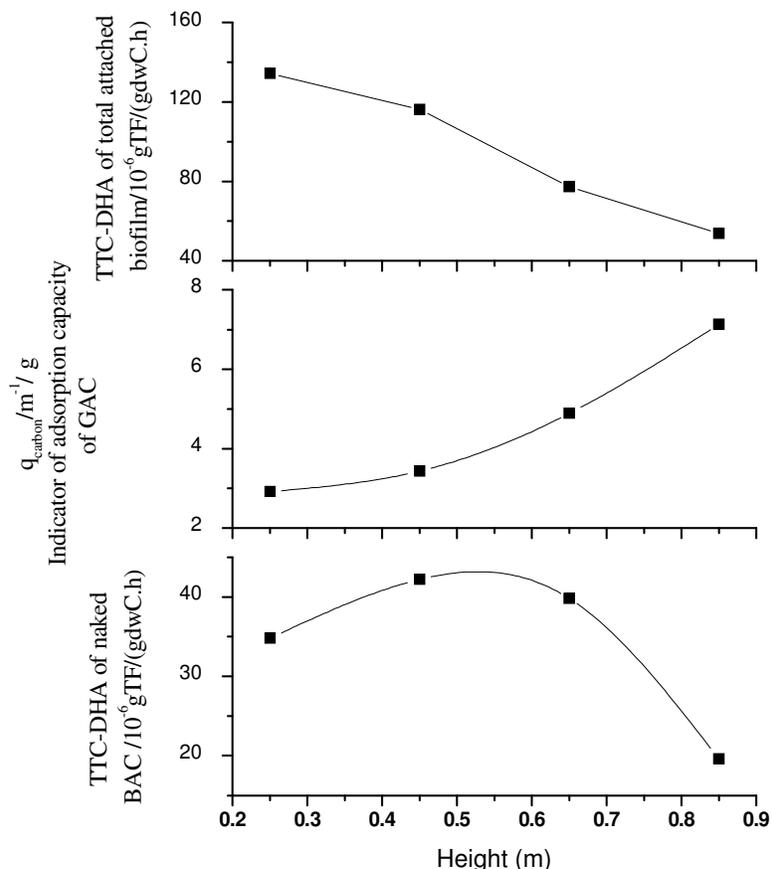
**Figure 5.** Multi-relations of GAC adsorption capacity, TTC- DHA activities of the naked BAC samples and corresponding TTC- DHA activities of attached biofilm changing with the height of biofilter.
