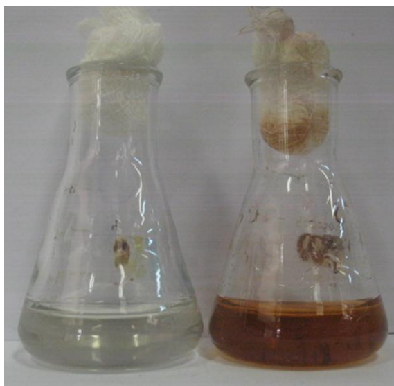
Figure 2. Photograph of reductase before (left) and after (right) complete reaction with silver nitrate.
