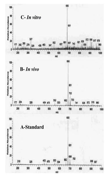
Figure 6. LC-ESI-MS analysis of *in vivo* and *in vitro* grown tubers with standard. A, Standard; B, *In vitro*; C, *in vivo*.
