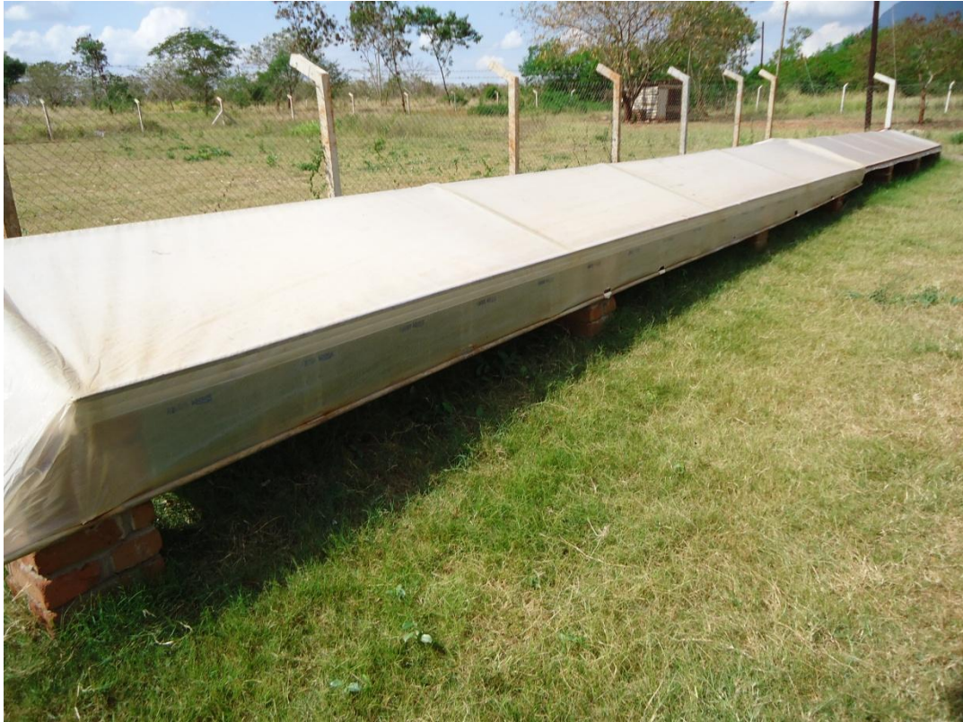
Figure 3. Tunnel solar dryer covered after placing samples for drying.
