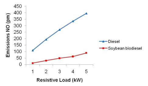
Figure 3. Means of NO emissions for both fuels in different resistive loads.
