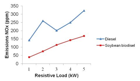
Figure 4. Averages of NOx emissions of both fuels for different resistive loads.
