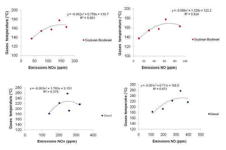
Figure 5. Correlation between gases exhaust temperature and NO and NOx emissions.
