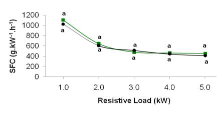
**Figure 1.** Specific fuel consumption according to the applied load. Treatments averages followed by different letters significantly differ from each other by Tukey's test at 5% of significance.
