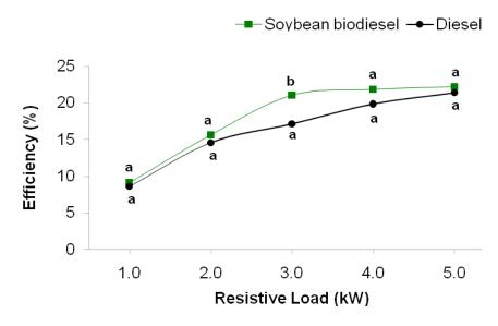
**Figure 2.** Efficiency of the engine-generator set in converting the fuel's chemical energy into electric energy. Treatments averages followed by different letters significantly differ from each other by Tukey's test at 5% significance.
